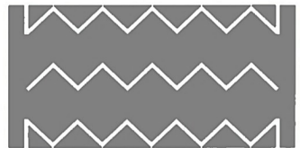
Zigzag lines found on the side of pedestrian crossings: No parking, waiting or overtaking
