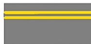
Double yellow lines: depicts the side of the carriageway, no parking or stopping
