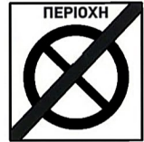
End of no parking zone with limited duration
