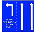
With-flow bus lane which other vehicles can use to turn left
